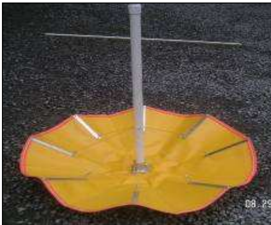
Fully Opened Debris Dam
